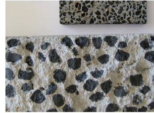
Beads acting as lightweight concrete aggregates
