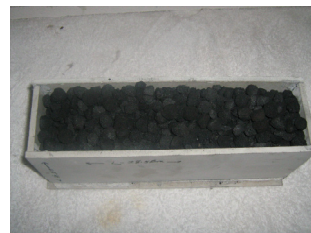
Cavity filled with loose insulation made up of carbon beads
